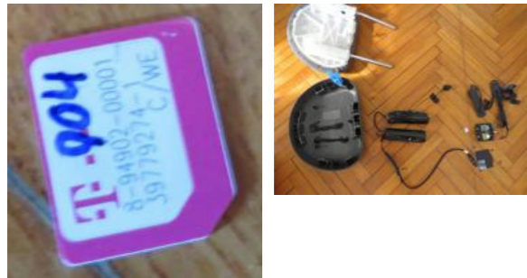
1: control unit; 2: batteries; 3: GPS antenna; 4: micro-phones connected to the listening device; 5: SIM card 6: dismantled listening device; 7: SD card
