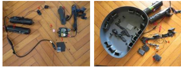
1: control unit; 2: batteries; 3: GPS antenna; 4: micro-phones connected to the listening device; 5: SIM card 6: dismantled listening device; 7: SD card
