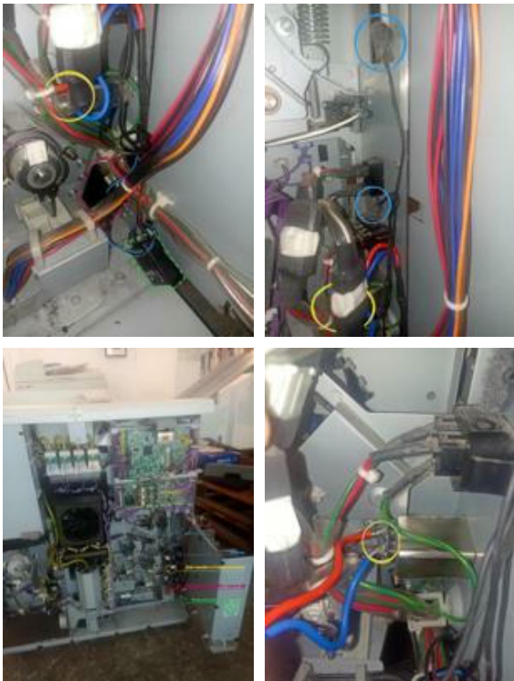
Blue: microphones; yellow: wires soldered to the power supply; pink: small box with SIM card + SD card; green: transformer.
