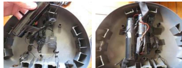
1: control unit; 2: batteries; 3: GPS antenna; 4: micro-phones connected to the listening device; 5: SIM card 6: dismantled listening device; 7: SD card
