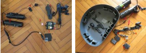
1: control unit; 2: bat- teries; 3: GPS antenna; 4: microphone; 5: SIM card. 2: the two batteries of the listening device; 4: microphones con- nected to the listening device; 6: dismantled listening device; 7: SD card.
