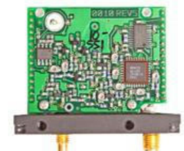
Module providing RF transmission capabilities
