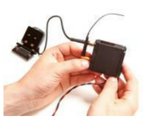
Transmitter-receiver module (closed)
