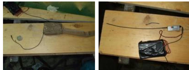
The device was like that when it was found. The microphone is next to the two euros coin and the antenna is at the other end.
