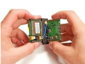
Transmitter-receiver module (open)
