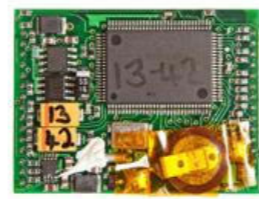
Module providing the GPS signal (other side)
