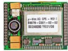
Module providing the GPS signal
