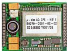
Module providing the GPS signal
