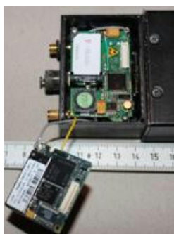
GPS tracker open with SIM card
