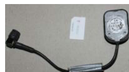
GPS antenna and SIM card
