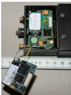
GPS tracker open with SIM card
