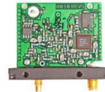
Module providing RF transmission capabilities
