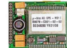
Module providing the GPS signal
