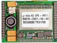
Module providing the GPS signal
