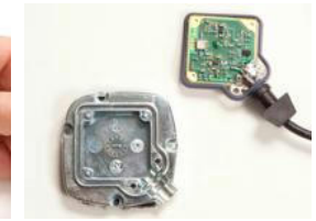
GPS antenna board
