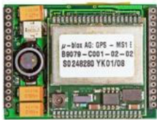
Module providing the GPS signal
