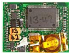
Module providing the GPS signal (other side)
