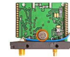
Module providing RF transmission capabilities (other side)
