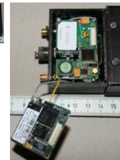
GPS tracker open with SIM card
