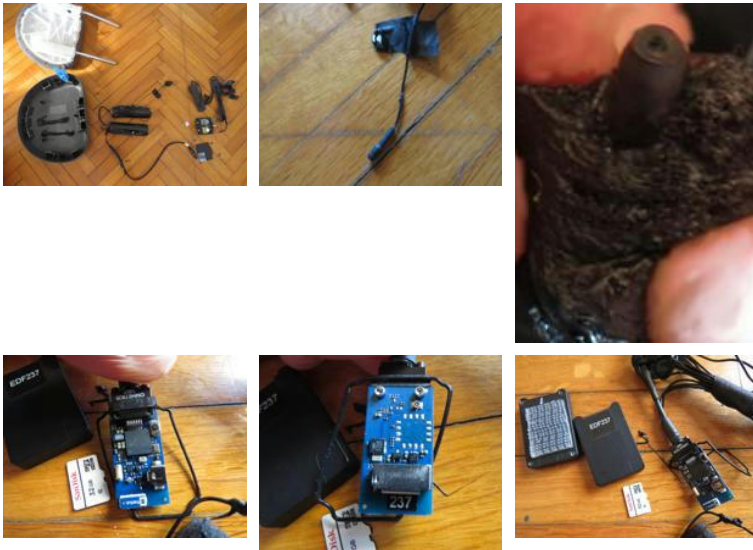
1: control unit; 2: batteries; 3: GPS antenna; 4: listening device; 5: microphones connected to the listening device; 6: dismantled listening device; 7: SD card
