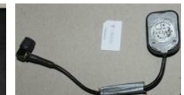
GPS antenna and SIM card
