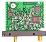
Module providing RF transmission capabilities
