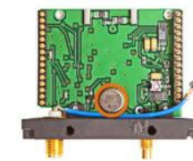
Module providing RF transmission capabilities (other side)
