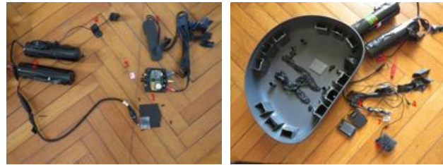
1: control unit; 2: batteries; 3: GPS antenna; 4: microphone; 5: SIM card; 6: microphones connected to the listening device; 7: dismantled listening device; 8: SD card
