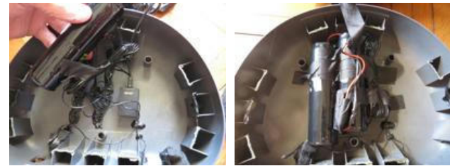
1: control unit; 2: batteries; 3: GPS antenna; 4: microphone; 5: SIM card; 6: microphones connected to the listening device; 7: dismantled listening device; 8: SD card
