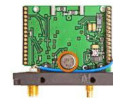
Module providing RF transmission capabilities (other side)
