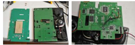
On the left: modified version of the phone largest circuit board (with surveillance device) without the battery pack. On the right: unmodified version. The phone smallest circuit board, with added wiring to allow recording of audio by the surveillance device on the other circuit board.
