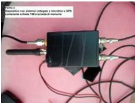
The device with an antenna connected to the microphones and the GPS. It also included a SIM and memory card.
