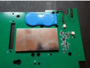
Modified version of the phone’s largest circuit board (with surveillance device). The battery pack (in blue) and the shielded module (in light brown) are part of the surveillance device.
