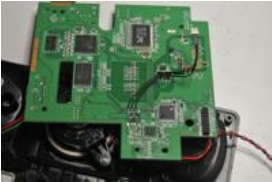
The phone’s smallest circuit board, with added wiring to allow recording of audio by the surveillance device on the other circuit board.
