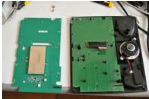
On the left: modified version of the phone’s largest circuit board (with surveillance device) without the battery pack. On the right: unmodified version.
