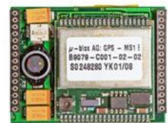
Module providing the GPS signal
