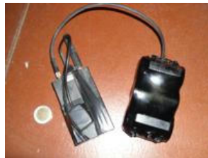
Counterclockwise from top: device with antenna, SIM and memory card; GPS; power cables.
