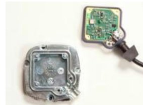
GPS antenna board
