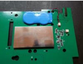
Modified version of the phone’s largest circuit board (with surveillance device). The battery pack (in blue) and the shielded module (in light brown) are part of the surveillance device.
