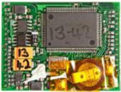
Module providing the GPS signal (other side)
