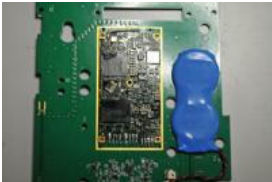
Modified version of the phone’s largest circuit board, with the cover of the shielded module removed.
