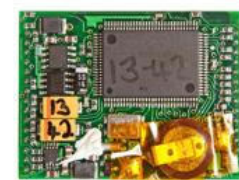
Module providing the GPS signal (other side)
