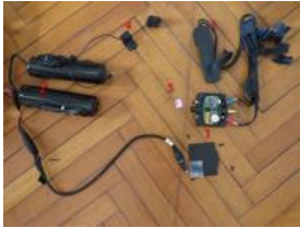
1: control unit; 2: batteries; 3: GPS antenna; 4: listening device; 4: microphones connected to the listening device; 6: dismantled listening device; 7: SD card
