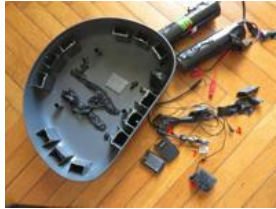
1: control unit; 2: batteries; 3: GPS antenna; 4: listening device; 4: microphones connected to the listening device; 6: dismantled listening device; 7: SD card
