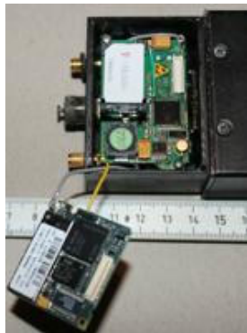
GPS tracker open with SIM card
