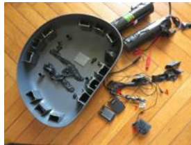
2: the two batteries of the listening device; 4: microphones connected to the listening device; 6: dismantled listening device; 7: SD card.
