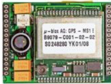
Module providing the GPS signal
