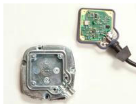
GPS antenna board
