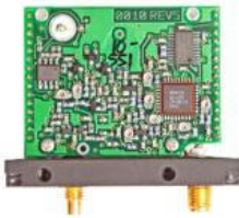
Module providing RF transmission capabilities
