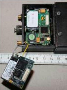
GPS tracker open with SIM card
