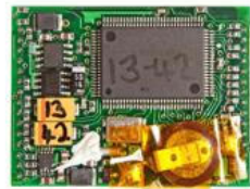
Module providing the GPS signal (other side)
