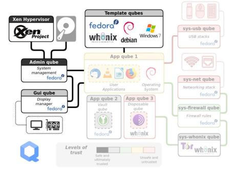
Two more components are needed to complete the Qubes OS system:
