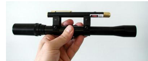
Simple laser / rifle scope system.
