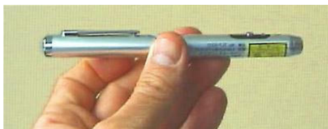
Inexpensive laser pointer (1 mW, 650 nm red).
