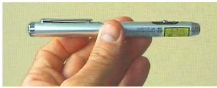
Inexpensive laser pointer (1 mW, 650 nm red).
