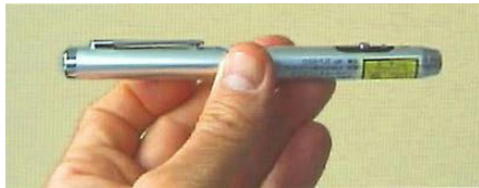
Inexpensive laser pointer (1 mW, 650 nm red).
