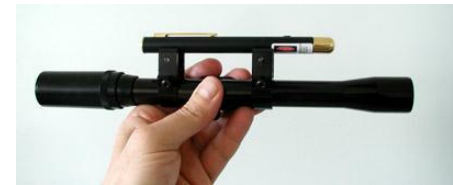
Simple laser / rifle scope system.
