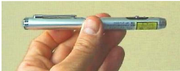
Inexpensive laser pointer (1 mW, 650 nm red).
