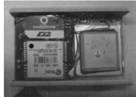
Inside view of a GPS tracking module. At the top left the GSM card for transferring data via cellular network.
