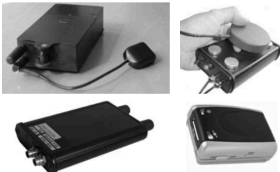
Four classic or commercially available GPS tracking modules from the years 2007–2009.
