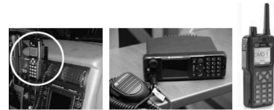
TETRA devices currently in use: hand-held device permanently installed in the car; MRI (base unit) from Motorola; HRT (hand-held) from Sepura.
