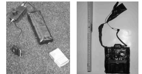
Left: GPS transmitter from the LKA Schleswig-Holstein (2007), GPS antenna and battery set separately.
