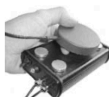
Right: GPS transmitter from the BKA (2007), GPS antenna separately.
