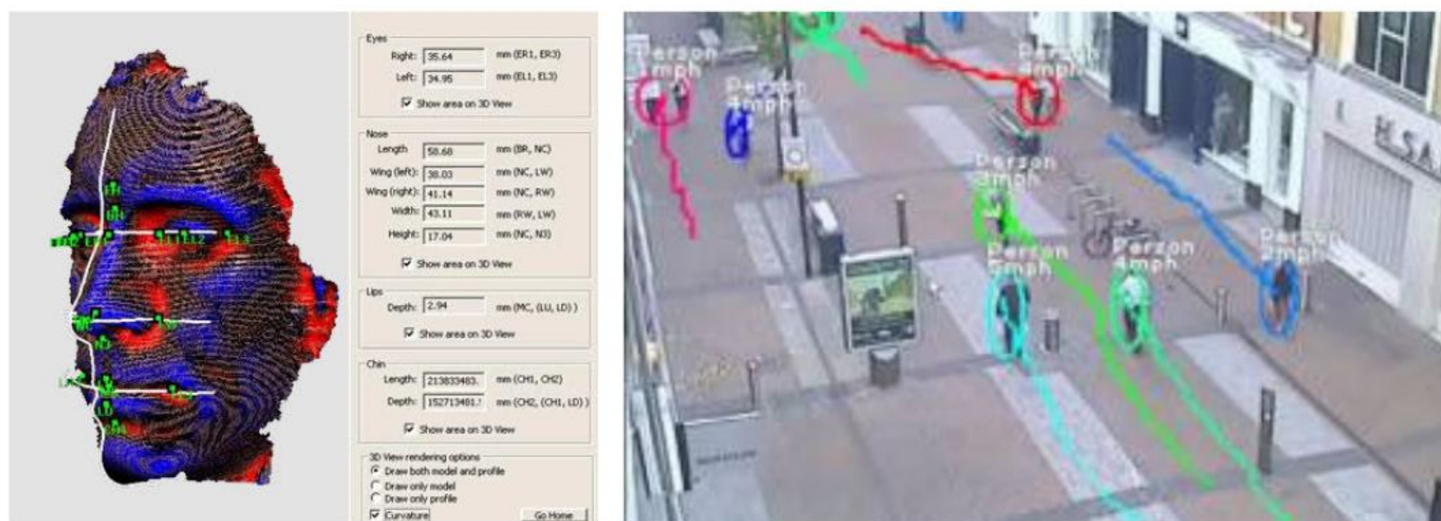
(LEFT) EXAMPLE OF FACIAL RECOGNITION SOFTWARE MAPPING BIOMETRIC MEASUREMENTS. (RIGHT) 'SMART CCTV' CAMERA FOOTAGE, TRACKING MULTIPLE MOVING TARGETS.
