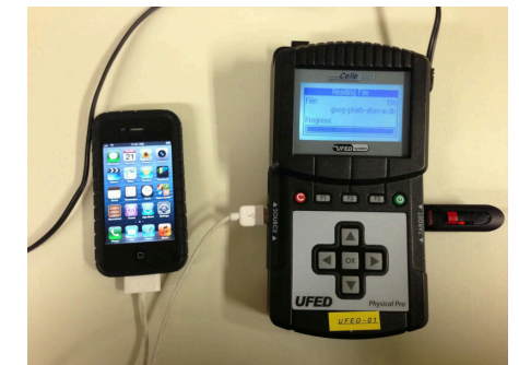
A Cellebrite Universal Forensics Extraction Device (UFED) extracting data from an iPhone 4S, 2013.
