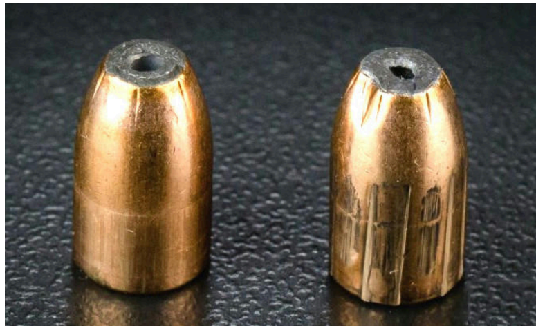
On the left, an unfired 9mm bullet. On the right, a fired bullet of the same model.
